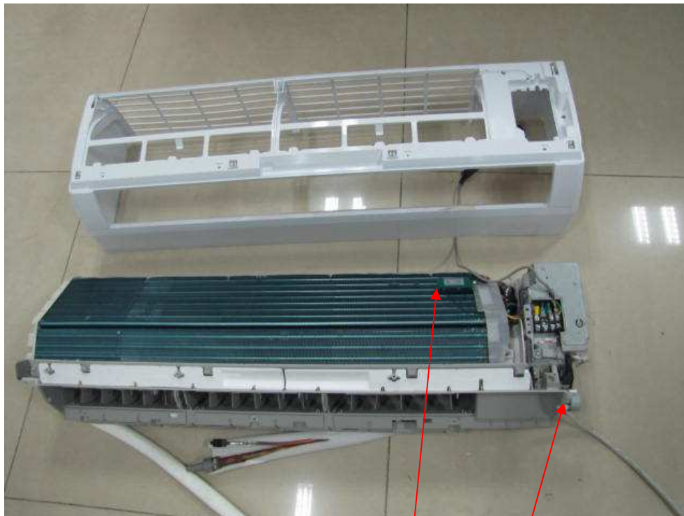
Internal view (location of Cold Plasma Generator, swing fan motor)
