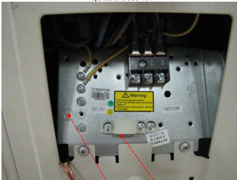
Internal view (earthed marking, cord anchorage)
