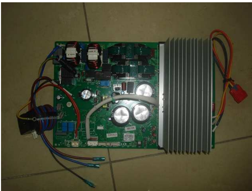
Main board W8603E with electrical heat belt
