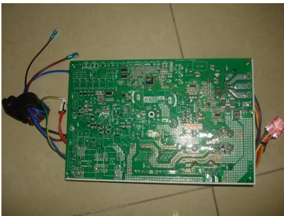
Main board W8603E with electrical heat belt
