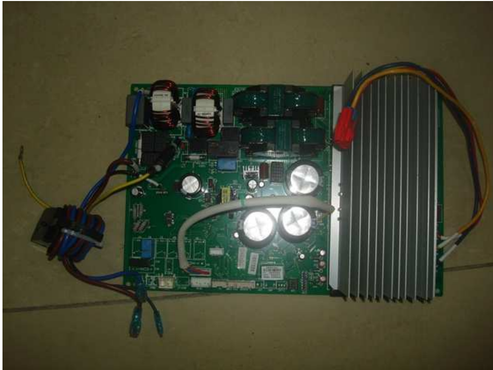
Main board W8602B without electrical heat belt
