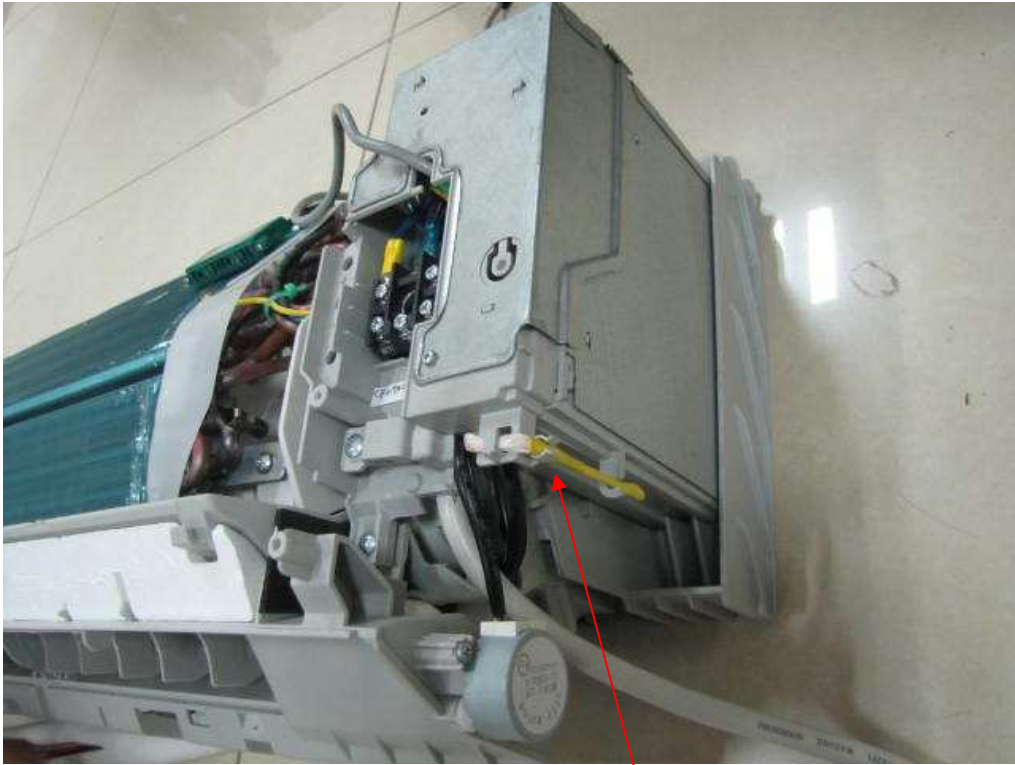
Internal view (location of temperature sensor)
