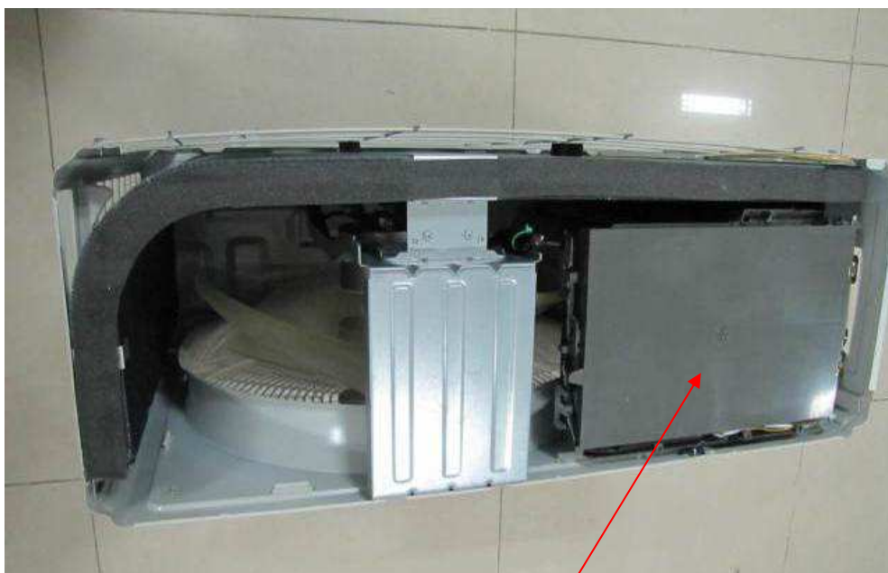
Open top cover view (main PCB box)
